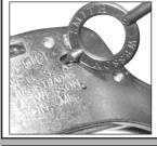
Insert the small peg on the top of the key into the double lock slot. In this position, the small peg can contact the end of the lock spring. Slide the key toward the key hole. This causes the lock spring to move into a position that locks the bolt thus preventing the cuff from being further tightened.
